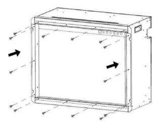
**5.** Put the appliance into the wall opening and fix it with the screws provided.
