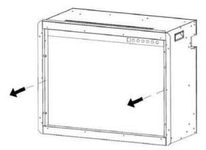
**4.** Place the left, right, top, and bottom trims on the appliance and fix the part using the screws provided in the kit.
