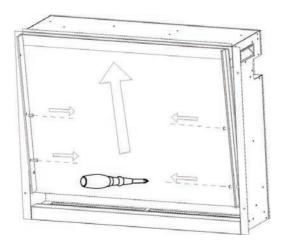
3. Install the fireplace into the wall opening. Fix the FOUR wall screws in each side of the fireplace box.
