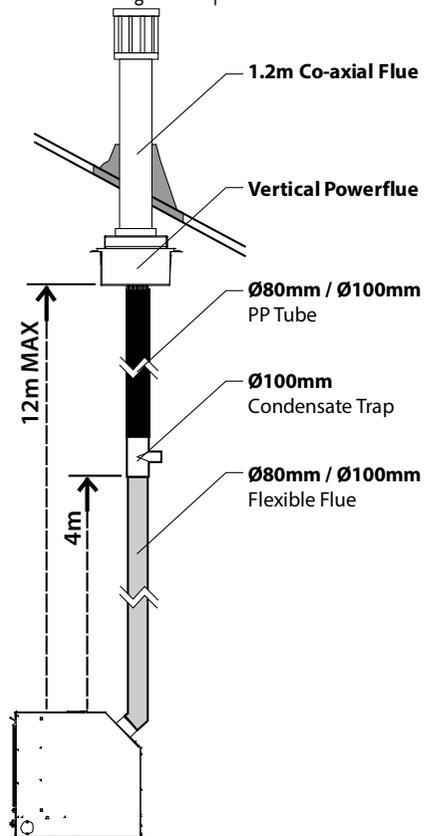
**Vertically Terminated:** Utilises the Escea vertical power flue enclosure kit.
