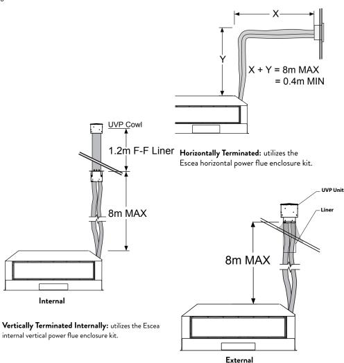
**Vertically Terminated Externally:** utilizes the Escea external vertical power flue enclosure kit
