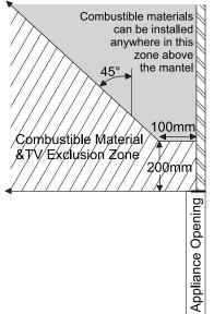
For DF700 & DF960 the minimum height for TV installation without a mantel installed: 200mm
