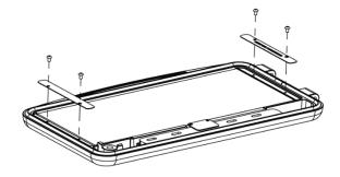
2) Take out the glass, and check if the grey rope beneath needs replacing. If so, replace this rope as well.
