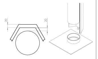
3) Solid Flue Shield – a full length, solid outer flue shield (7.75" – 8" diameter) extending from the heater through into the drop box penetrating the ceiling. The base of the solid outer shield must be fitted with the Decromesh Locating Ring supplied with in the heater.
