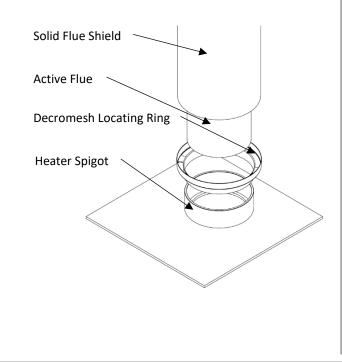
4) Decromesh – a full length, half radius perforated Decromesh flue shield (7.75" – 8" diameter) extending from the heater through into the drop box penetrating the ceiling. The base of the decromesh must be fitted with the Decromesh Locating Ring supplied with in the heater.
