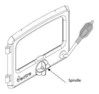
A tool for opening and closing the air spindle is supplied with the heater. This can be used in instances when the spindle control is too hot to touch. Alternatively, a glove or equivalent can be used to adjust the air spindle.
