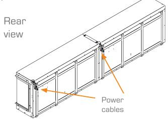
This model requires 2x power points and a total of 13.04 Amps and therefore may require it's own circuit. It is recommended that for an optimum installation it is hard wired with it's own circuit.
