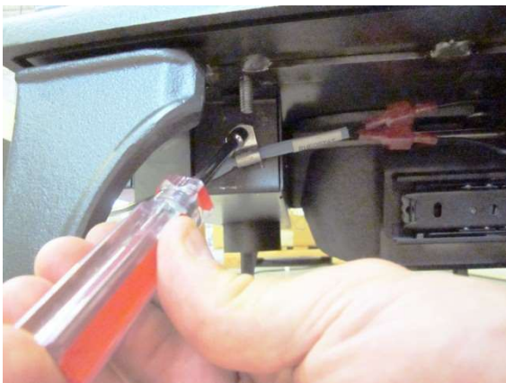
Cape Cod / Rockport Wire Clamp Location
