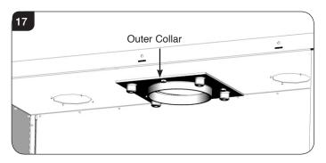
11.7 There is a Flue Collar Bracket on top of the Outer Box. This locates on two pins that allow flexibility when replacing the Outer Collar. The bracket remain in place when installing the flue system, see Diagram 18.
