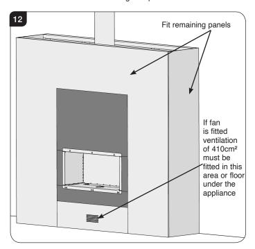
If a convection fan is to be fitted, leave a convection hole in the lower panel below the front of the opening. This hole must have a minimum free area of 410cm².
