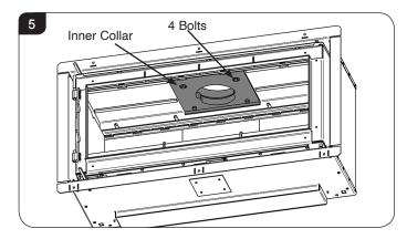
5d.2 The 2 x longer front bolts are recessed into the collar, see Diagram 9.
