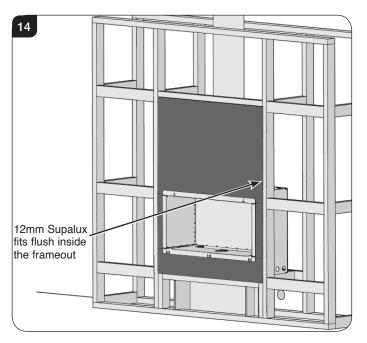
9.5 Fit another layer of Heat Resistant Board to the highlighted area ensuring it is at least 400mm to the sides and 900mm above the appliance.
