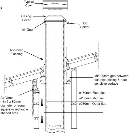
Note: All external air vents & ceiling penetrations must be bird & rodent proofed with permanently fixed screens
