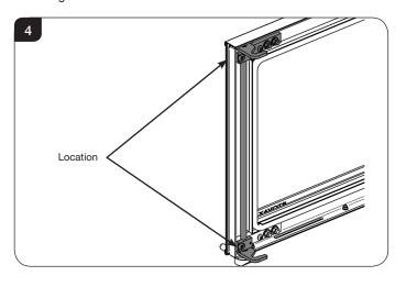
6a.3 The top and bottom catches will need to be adjusted separately and in the same manner. The catch block can move in two directions, see Diagram 5, 6 & 7.
