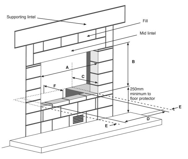
Many fireplace openings have a supporting lintel. Remove the covering plaster to identify its position before starting any constructive work. Do not remove constructional lintels without making provision to support the remaining structure of the building. The appliance must not form any part of the supporting structure.
