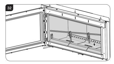
— Slide the Log Guard across so both end locate evenly in the holes in the side bricks, See Diagram 33.
