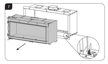
Pull the inner box carefully forward to release from the cutouts. It should now slide smoothly out of the outer box.
