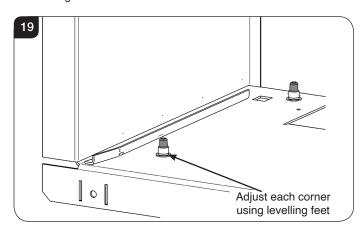
11.11 Wind the set screws down to the desired position in each corner.
