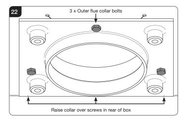
12.2 To ensure the outer collar is central, and **to avoid cross threading of the bolts** during actual installation, feed the 4
