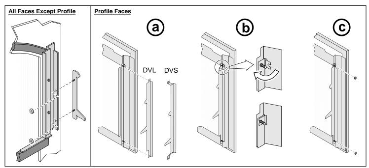
6 The face mounts to the brackets as shown in the illustration below.
